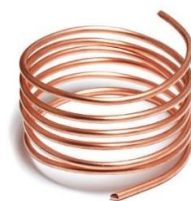
Ductile Ability to be stretched into a length without breaking
